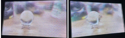
Fig. 6 A set of elemental image with 46° viewing angle in Experiment 1
